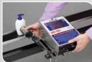
**Step 2:** Slide the compact printer on to the mounting bracket and adjust the print head to your product.
