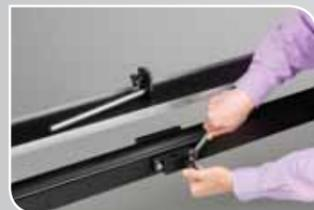
**Step 1:** Simply drill two holes to fit the sturdy mounting bracket to your conveyor.
