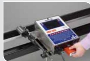
**Step 3:** Push the sealed ink cartridge into the printer, and connect a power supply.
